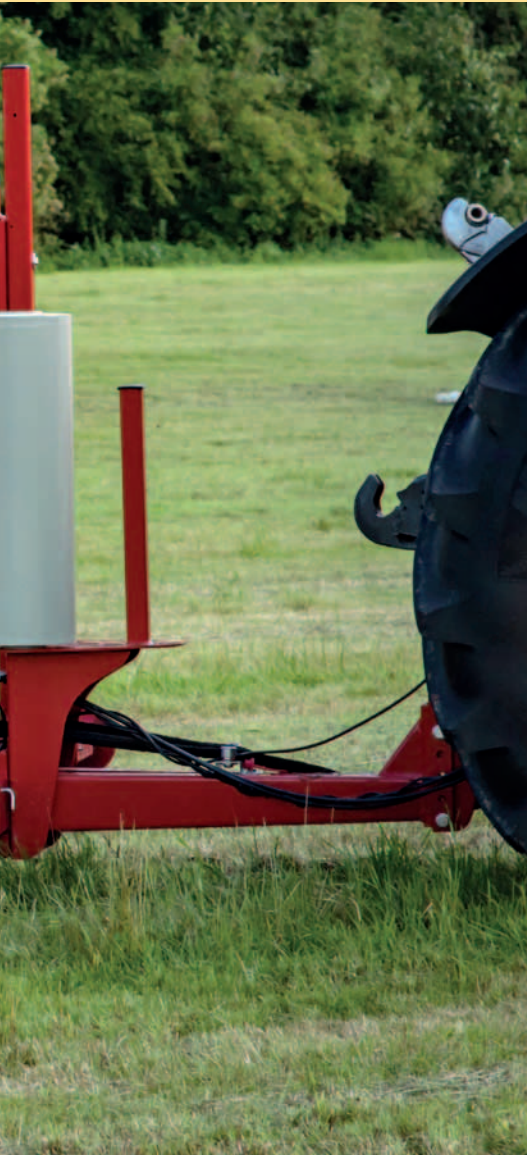
To achieve a narrower transport width, the right hand wheel is turned to the inside of the support arm.
